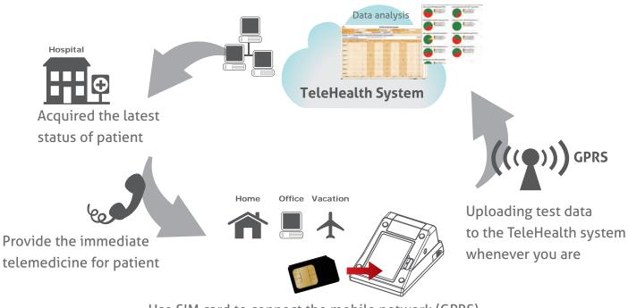
Use SIM card to connect the mobile network (GPRS)
