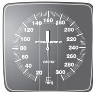
Gauge properly set to zero square position
