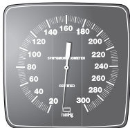
Gauge out of zero square position
