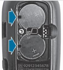
Slide the new batteries under the black tabs and
