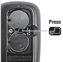
Release the old batteries by pressing the
