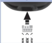
Insert the test strip into the meter in the direction of the arrows.
