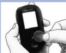
Remove the old battery and place the new one in the meter with the **(+)** side facing up.
