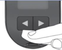
Turn the meter off and wipe the entire meter surface with a Super Sani-Cloth. Carefully wipe around the test strip slot and other openings.
