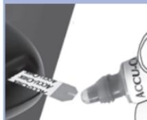
Touch the drop to the **front edge** of the yellow window of the test strip until you see flash. **Do not put control solution on top of the test strip.**
