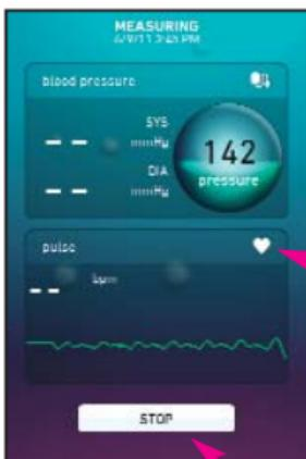
3. The module automatically pumps up the cuff. Remain at rest during the reading: do not move and do not talk.
