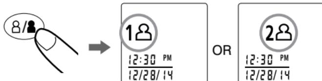
2. Press and hold the **DATE/TIME SET ⊖ and + buttons** at the same time while in memory recall mode and the data for the selected user will be erased automatically.
