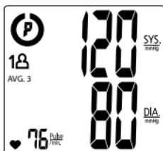
5. Every new press of the **M button** will recall a previous reading. The latest reading will be recalled first.
