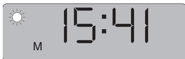
Fig. 3-6 Example: display after successful self-test ( M = BP data in memory, ☀ measuring phase: day)
