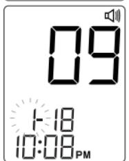
With the day flashing, press **▲** or **▼** until the correct day appears. Press **S**.
