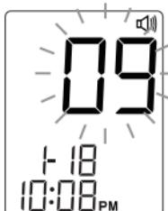
With the month flashing, press **▲** or **▼** until the correct month appears. Press **S**.
