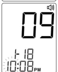
With the minute flashing, press **▲** or **▼** until the correct minute appears. Press **S**.
