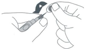
4. Replace the cap by aligning the arrow on the cap with the release button.
