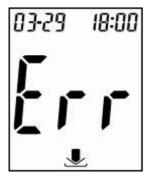
**Humidified/Used strips** *Action:* Replace with a new strip.
