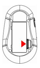
Put the battery door back in place and snap it closed. The meter turns on automatically.
