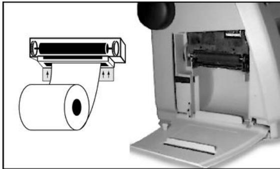
Any time the paper is loaded, the printer automatically prints a test strip with the DINAMAP<sup>®</sup> PRO name on it. If no print is visible on the paper, check that the paper roll has been installed in the correct position (refer to diagram). To tear off the printout, use a slight sideways action to pull the paper sharply up across the serrated edge of the door.
