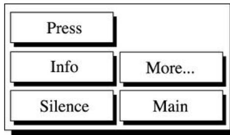
Press. Selection of this button displays a panel for setting the default BP target inflation pressure. Adjusting the default target pressure will automatically update the current inflation target pressure and will be used for the next reading. The range of adjustment is 100 mmHg to 180 mmHg, and the setting is retained when the Monitor is turned off.
