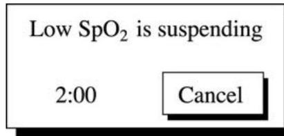
If the Monitor is unable to detect a pulse for 10 seconds during normal SpO<sub>2</sub> monitoring, the values in the LED flash, alternating patient values with dashes. The Monitor returns to normal SpO<sub>2</sub> reporting of values when several consecutive good pulse determinations are made.
