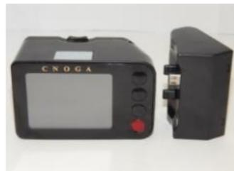
TensorTip turns on automatically when you initiate a measurement by closing the lid with your finger inserted, and turns off automatically 30 seconds after the last time any button was pressed. During a reading, the device will not turn off. You can also manually turn the device on by holding the On/Off button (
