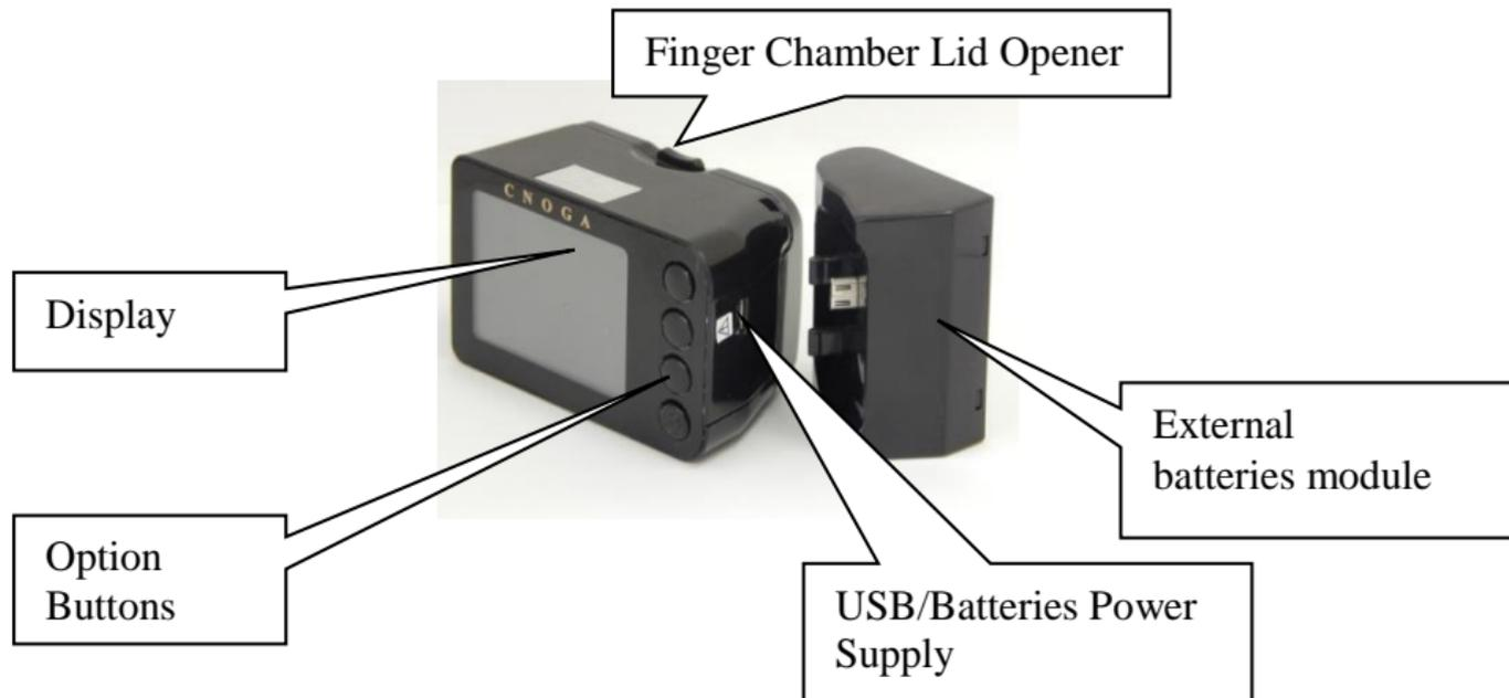
The Option Buttons change functionality depending on the status of the device as displayed on the screen. An icon on the screen indicates the function of each button. Push the adjacent option button to select the desired function.
