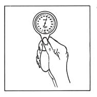
Place your thumb with light pressure on the Air Release button and observe the fall of pressure on the scale.
