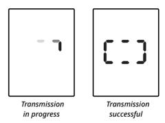
**18.** When the measurement has been successfully transmitted, the device shows the indication above before powering off.
