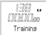
Once you are in the menu **Training**, your HR monitor automatically switches to the main display. This displays the already recorded training time on the middle line (after Save/Delete: 00:00:00) and on the line below **Start**.
