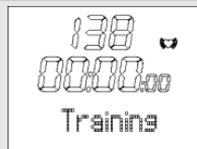
Once you are in the menu **Training**, your HR monitor automatically switches to the main display. This displays the already recorded training time on the middle line (after reset: 00:00:00) and on the line below **Start**.
