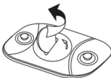
Remove the depleted button cell battery and insert a new button cell battery of the type CR2032. Ensure that the positive terminal (+) is facing upwards and the battery is positioned below the contact.
