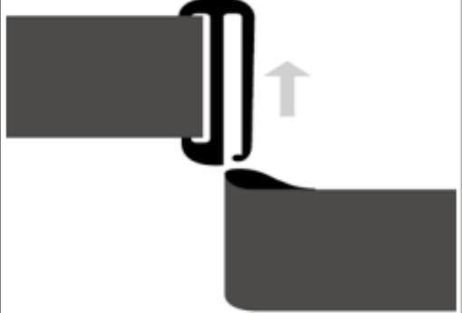
A diagram showing a dark grey chest strap with a black hook and loop fastener. A grey arrow points upwards from the hook, indicating it should be lifted to separate from the loop.                                 |
