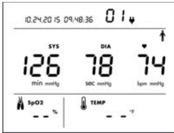
Example of SYS, DIA and HR* after BP measurement in Single Measurement Mode.
