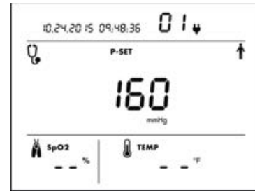
Example of Manual Mode display with cuff pressure at zero. P-set value is default 160 mmHg.
